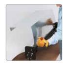
Accommodates sheet metal up to 48 in. (1.2 m) wide in any length. There is no fixed throat depth to contend with.
