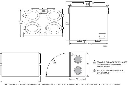
$VNT5150H1000, VNT5150E1000 \ or \ VNT6150H1000: \ H = 22 \ 1/2 \ in. \ (572 \ mm), \ W = 11 \ 1/2 \ in. \ (295 \ mm), \ L = 29 \ 1/2 \ in. \ (749 \ mm) \\ VNT5200H1000, \ VNT5200E1000 \ or \ VNT6200H1000: \ H = 22 \ 1/2 \ in. \ (572 \ mm), \ W = 16 \ 1/2 \ in. \ (422 \ mm), \ L = 29 \ 1/2 \ in. \ (749 \ mm) \\ M28919A$
